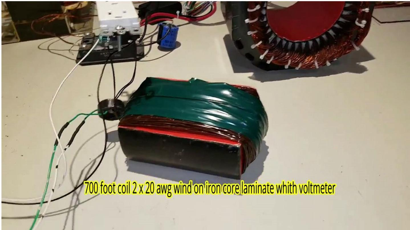
700 foot coil 2 x 20 awg wind on iron core laminate with voltmeter
