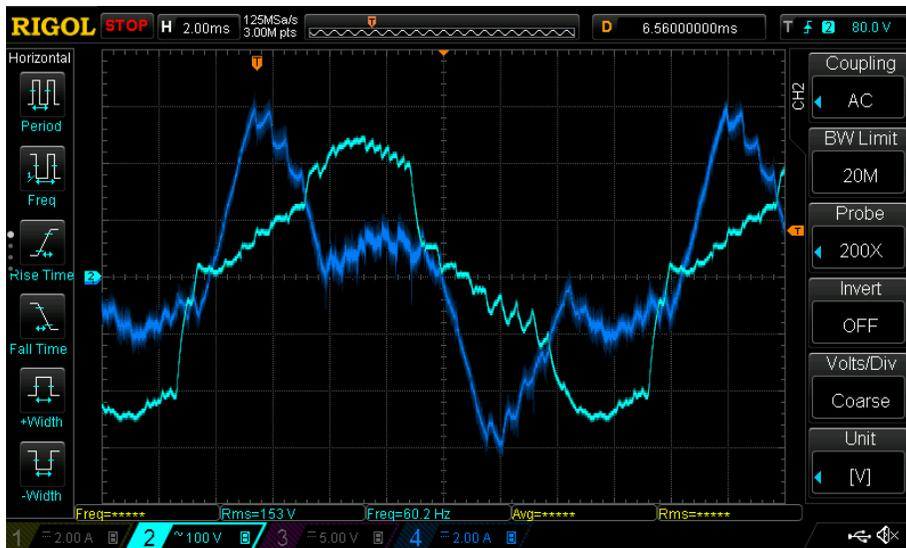
ttached is a slightly improved waveform, more symmetrical which produces a fairly good sine when filtered.
