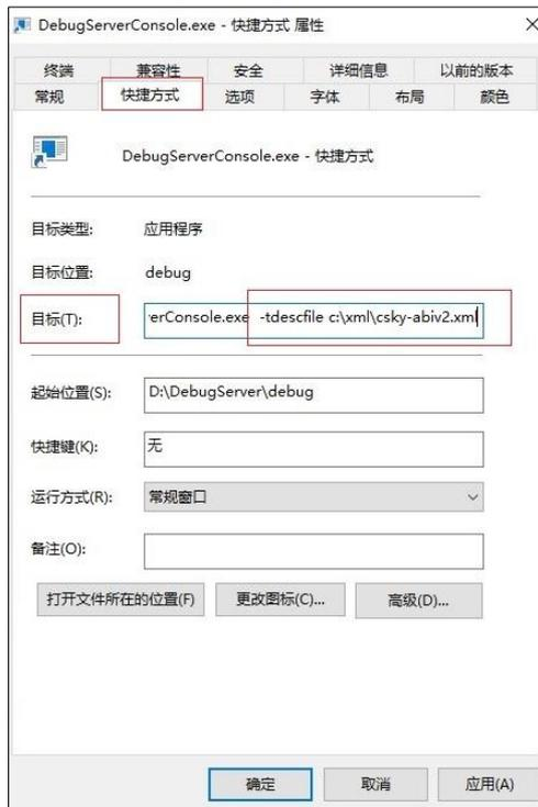
Figure 7-11-16 Clicking OK after modifying the startup parameter
