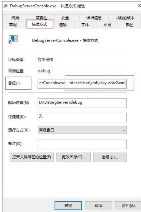
Figure 7-11-15 Add a startup parameter to the shortcut
